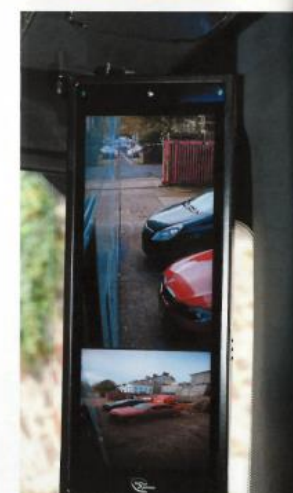
The buses have high-definition cameras relaying pictures to monitors inside the driver's cab instead of mirrors. ANDY IZATT
