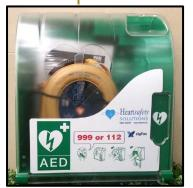
An IoT enabled AED storage cabinet that allows for remote monitoring has been developed. The cabinet is weather-proof and uses an optical sensor to view the AED screen, sending an alert as soon as there is a change in the status of the AED. In this way, an IoT solution maximises the efficiency of AEDs and potentially save lives.
