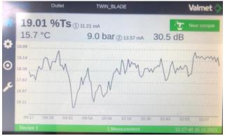
TS values after TS measurements calibration
