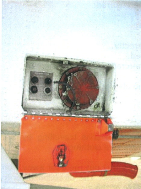
Pressure Refuelling Panel and Connection S61N.
