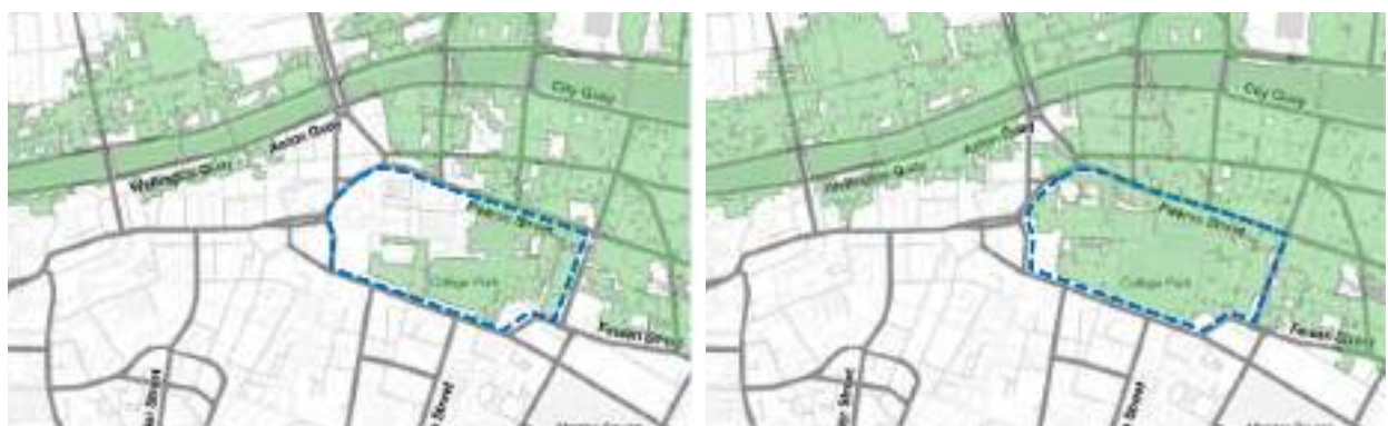
Figure 20. The main campus of TCD (blue dotted area) is at risk of coastal flooding under the mid-range-emission (20% increase in rainfall and 500mm rise in sea level; left) and high-emission scenarios (30% increase in rainfall and 1,000mm rise in sea level; right) (OPW, 2018a)
