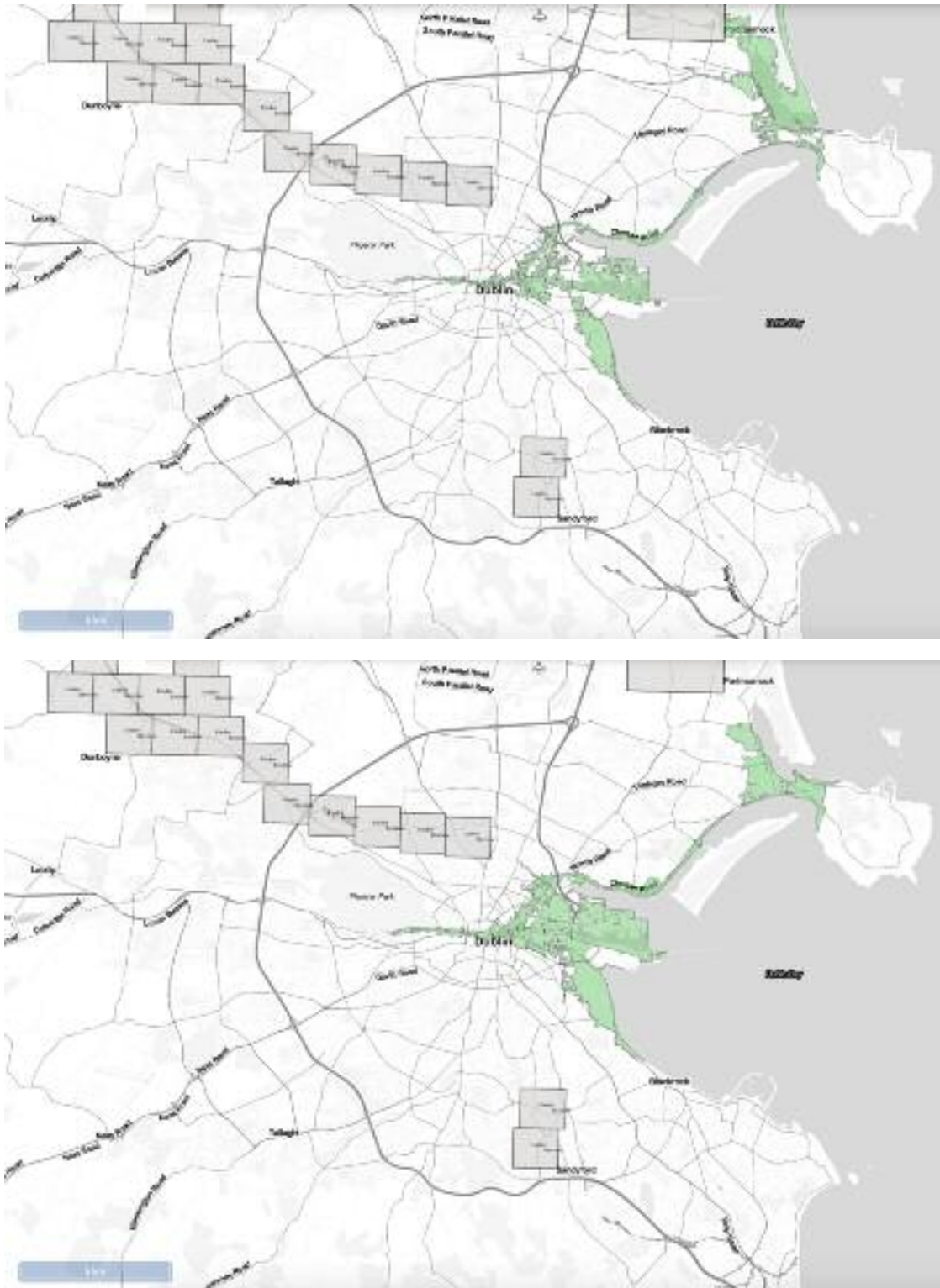
Figure 18. Future coastal flood extents in Dublin city based on a mid-range-emission scenario (20% increase in rainfall and 500mm rise in sea level, top) and high-emission scenario (30% increase in rainfall and 1,000mm rise in sea level, bottom) (OPW, 2018a)
