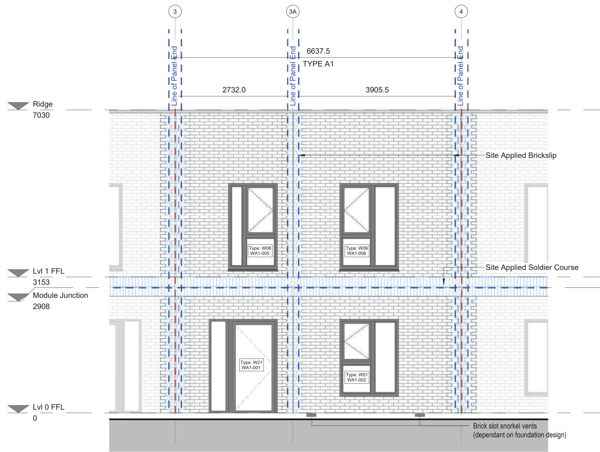
A1-F ELE-TYP-A1-FRONT ELEVATION-MID TERRACE 1:50
