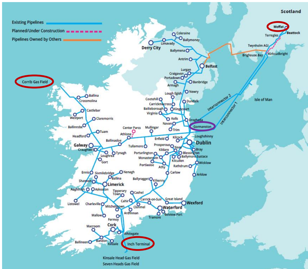
Figure 1: Overview of Gas Networks Ireland's Transmission System
