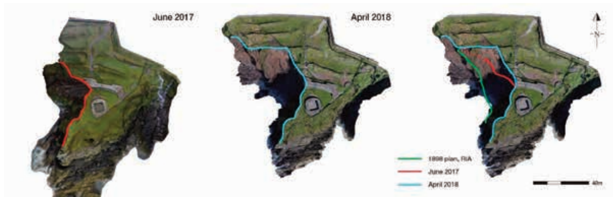
Figure 7. A 3D survey of Dunbeg Fort, mapping erosion from June 2017 (red line) through April 2018 (blue line). The green line indicates the coastline in 1898 (CHERISH, 2017, 2018).
