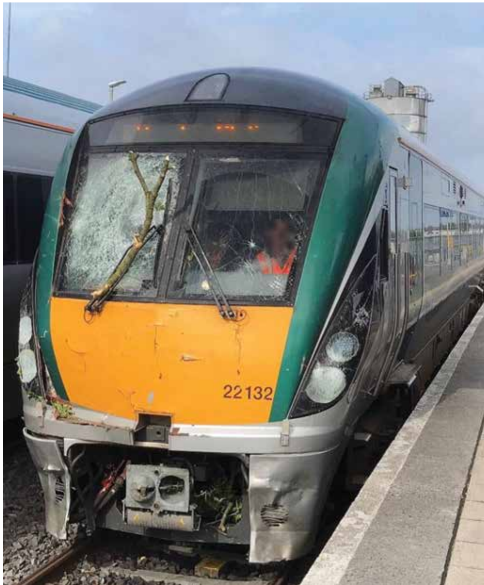
Figure 4.13: Train damaged by falling branches during Storm Ali, September 2018. Source: Irish Rail.
