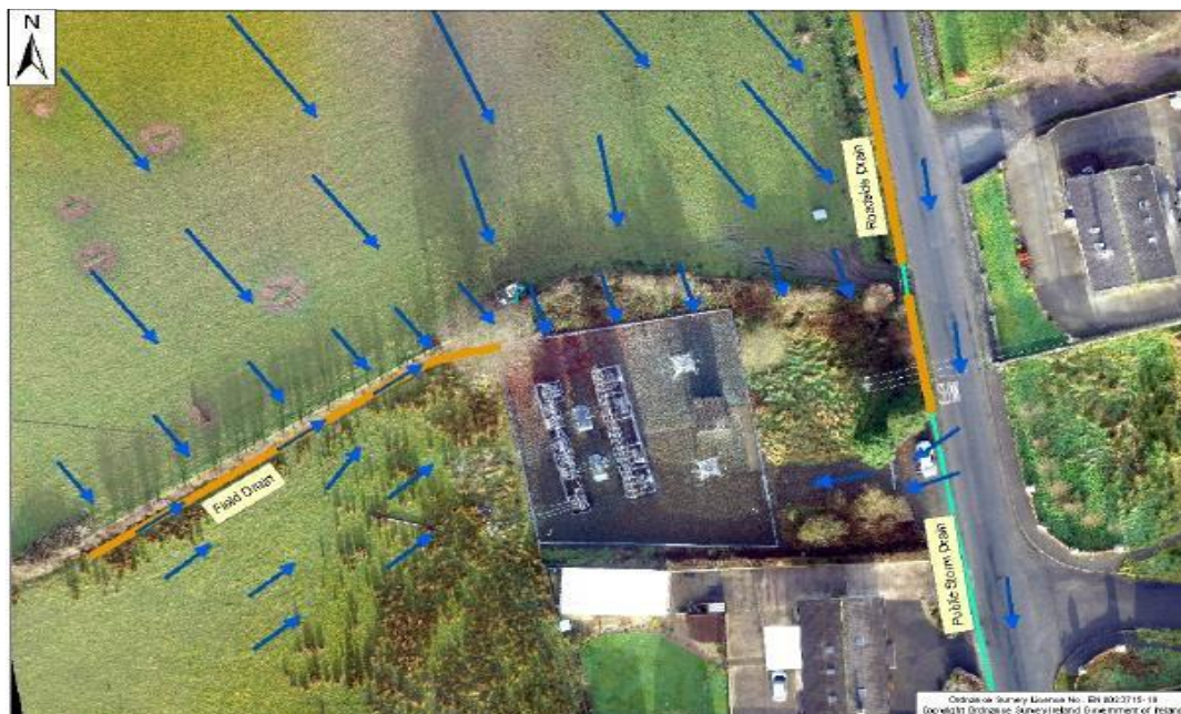
Figure 11 Flood routes into Station
