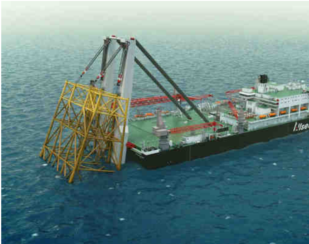
Figure 12: Specialist HLV, in this case, Pioneering Spirit, with jacket lifted from the seabed and tilted towards the vessel deck
