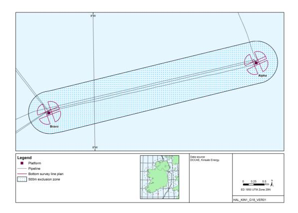
Figure 1: Provisional survey line plan around the Kinsale Alpha and Bravo platforms, including a 500m exclusion zone.
