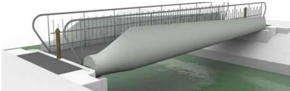
Fig. 1. Design for an 8 m span pedestrian/cycle bridge for greenways incorporating wind turbine blades
