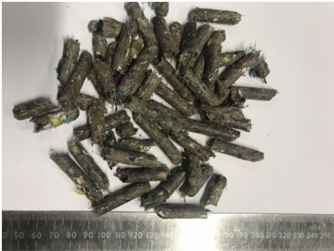
Figure 7 Highly Refined SRF Pellets developed by Beuparc
