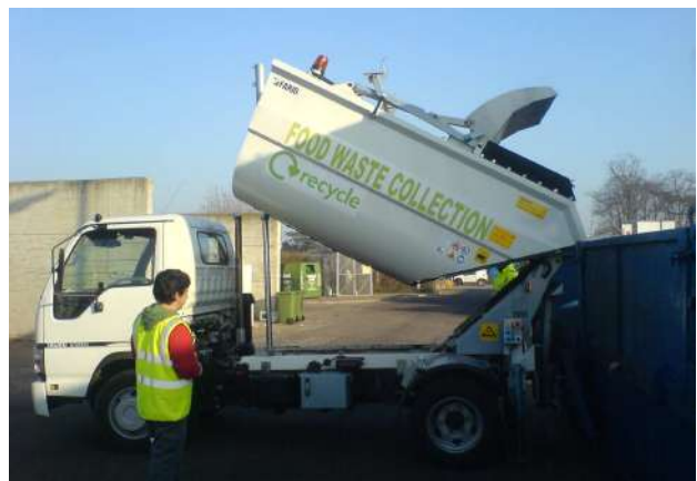
Localised bulking in Elmbridge – from vehicle directly into roll on off skip
