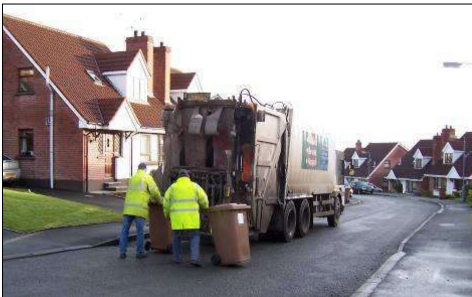
Figure 5: Collection of brown bin using mechanical loading into a packer truck in Armagh
