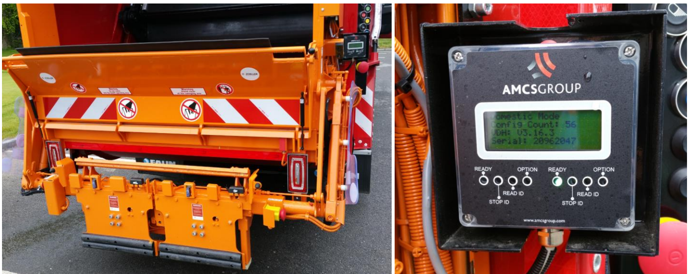
Photo 1 – Example of Weighing System on Refuse Collection Vehicle in Ireland
